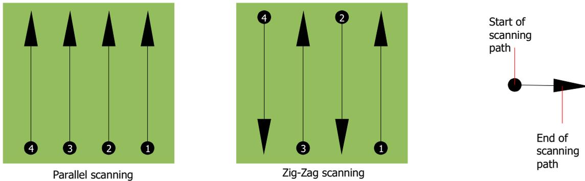
Figure 8.2: Scan modes to measure an area
