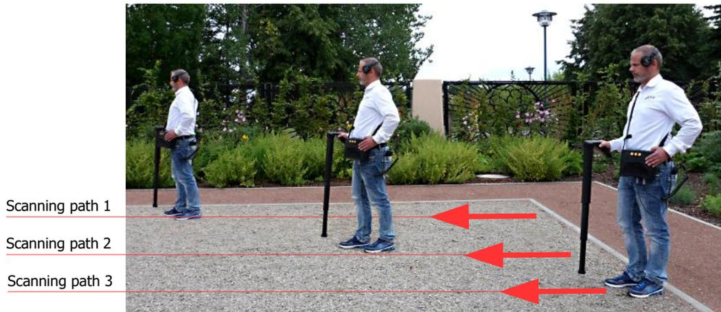
Figure 7.5: "Parallel" scanning in mode Ground Scan
