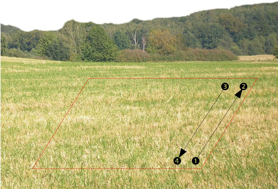
Figure 9.1: Measure area for a survey in mode "Ground Scan"
