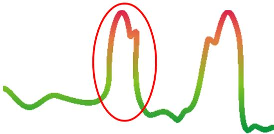
Figure 7.10: Signature of a non-ferromagnetic metal target
