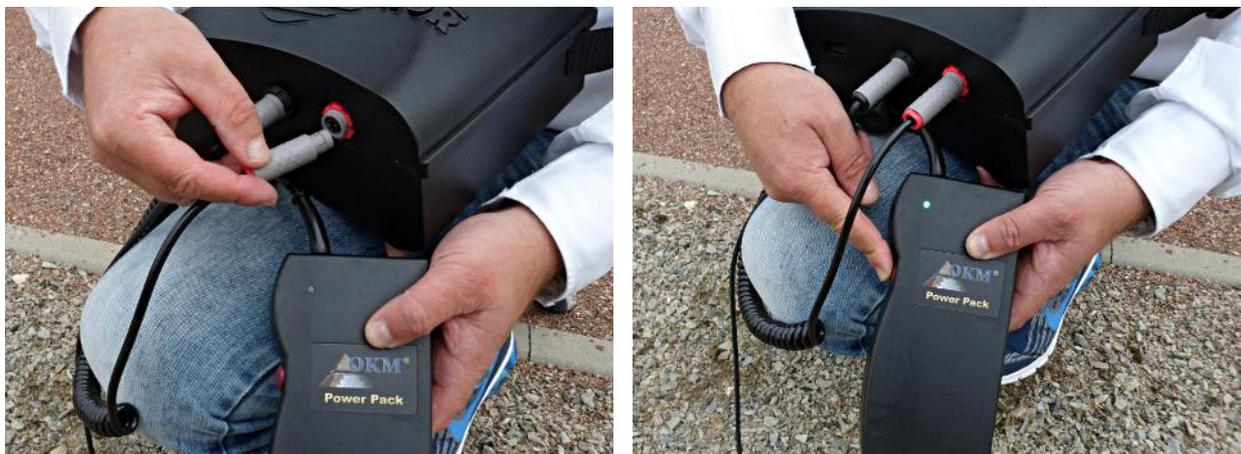
*Figure 6.10: Connecting the Power Pack (optional)*
