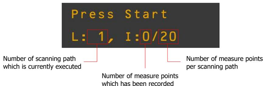
Figure 7.4: Display representation in operating mode "Ground Scan"
