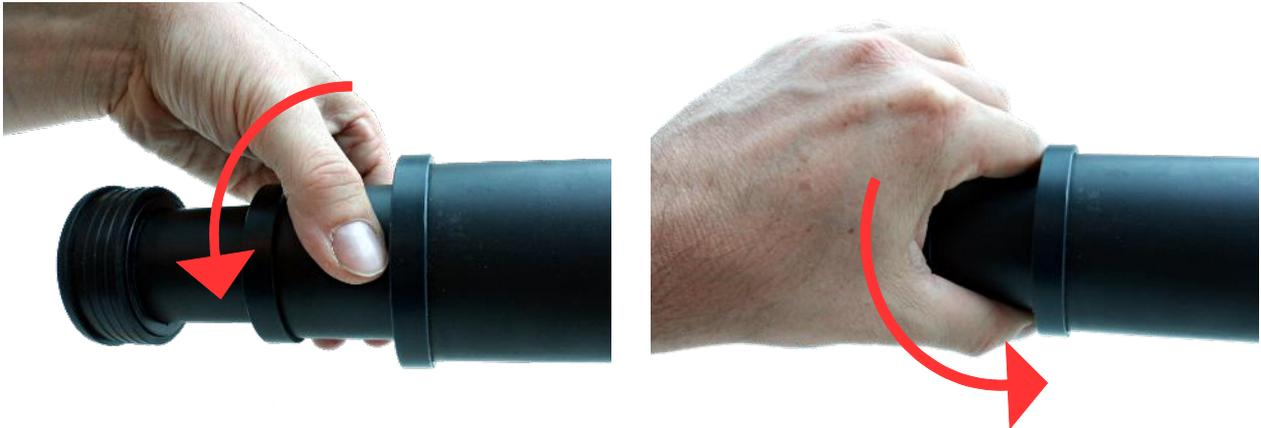
*Figure 6.3: Unlock the lower segments*
