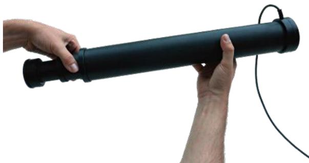
*Figure 6.2: Hold tight the upper segment, while extending the lower segments*
